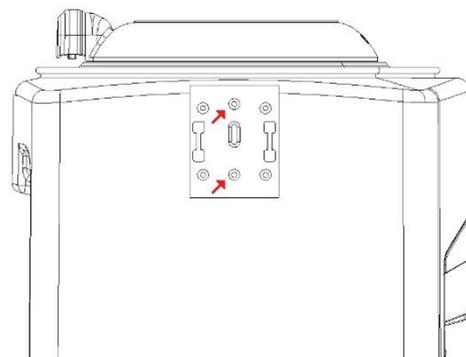
7. Slide the ADAM device onto the bracket. It will snap into position
